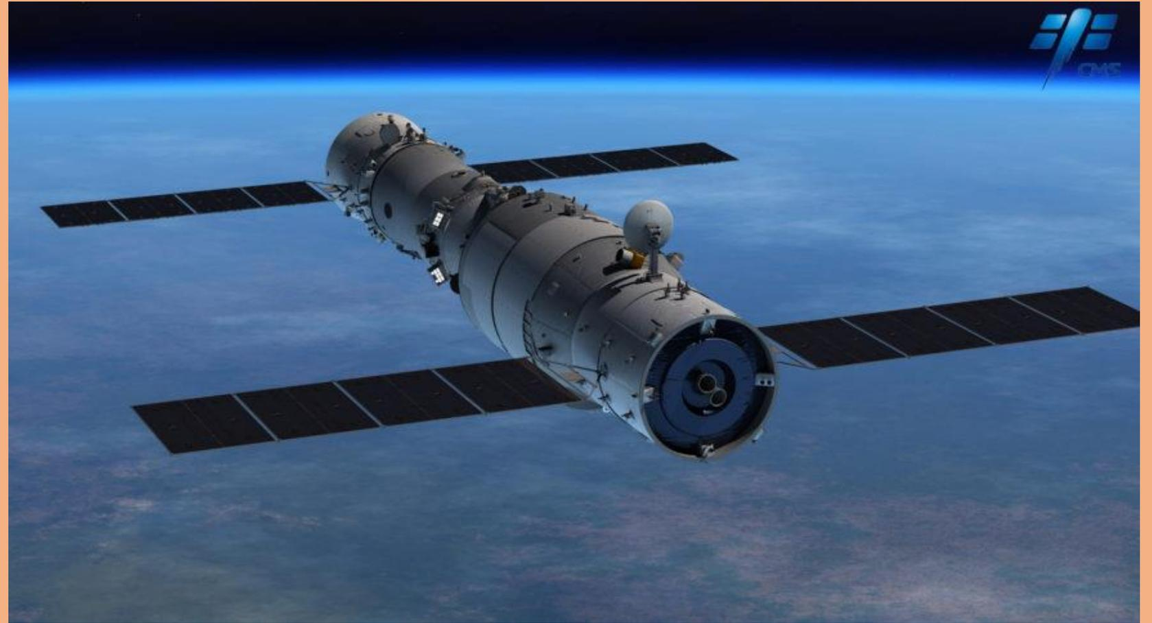
Tiangong-1 was China's first prototype [space station](#). It orbited Earth from September 2011 to April 2018, serving as both a manned laboratory and an experimental [testbed](#) to demonstrate [orbital rendezvous](#) and docking capabilities during its two years of active operational life.
