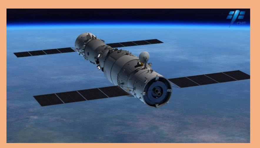
Tiangong-1 was China's first prototype <u>space station</u>. It orbited Earth from September 2011 to April 2018, serving as both a manned laboratory and an experimental <u>testbed</u> to demonstrate <u>orbital rendezvous</u> and docking capabilities during its two years of active operational life.
