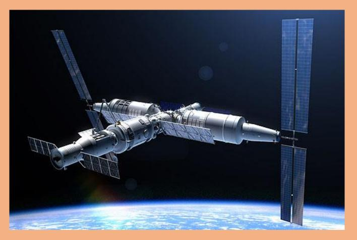
The central module called Tian He will be the first to be launched, from next year. It will serve as a place of life and work. Two scientific laboratories of about fifteen meters each will then be grafted to the station to form a pressurized volume of about 25% of that of the ISS. Once finalized, Tiangong 3 will be able to accommodate three Tikonauts for long-term stays in orbit.
